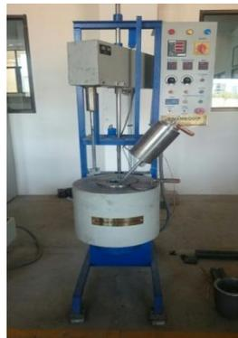
**Fig: 3** Stir Casting Equipment
