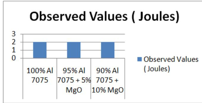
Fig:9. Graph Details of Impact Test
