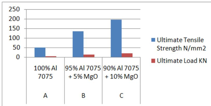
**Fig:8.** Graph Details of Tensile Test
