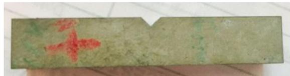
**Fig: 7** Impact Test Specimen
