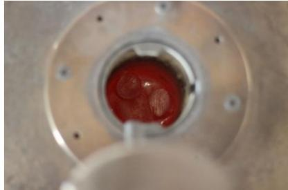
**Fig: 2** Melting of Al7075 in Stir Casting
