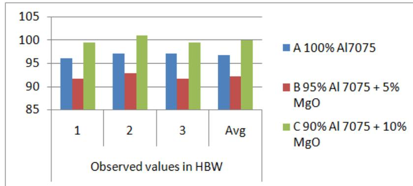
Fig:10. Graph Details of Hardness Test
